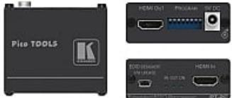
PT-2C is an EDID processor for 4K HDMI signals. It allows you to pass or block HDCP, multi-channel audio or deep color signals that may or may not be compatible with the display
